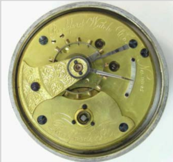
18s Model 1 full plate Key wind and key set Hunter #9845
