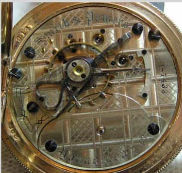
18s Model 3 full plate Stem wind and lever set Hunter Grade 40 #187433
