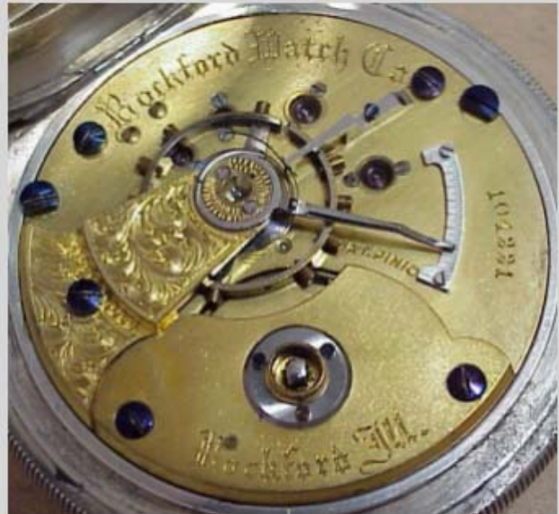
18s Model 2 full plate Key wind and lever set Hunter #104221
