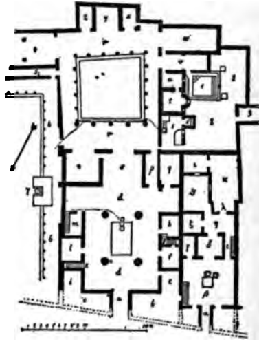
From Moss HOUSE OF THE SILVER WEDDING AT POMPEII Illustrating the Tetrastyle Atrium
